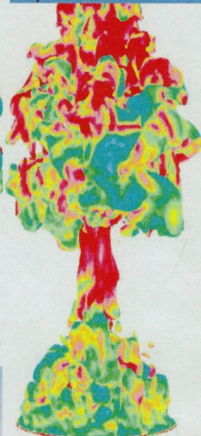
Snapshots of puff cycles showing isosurfaces of vorticity
