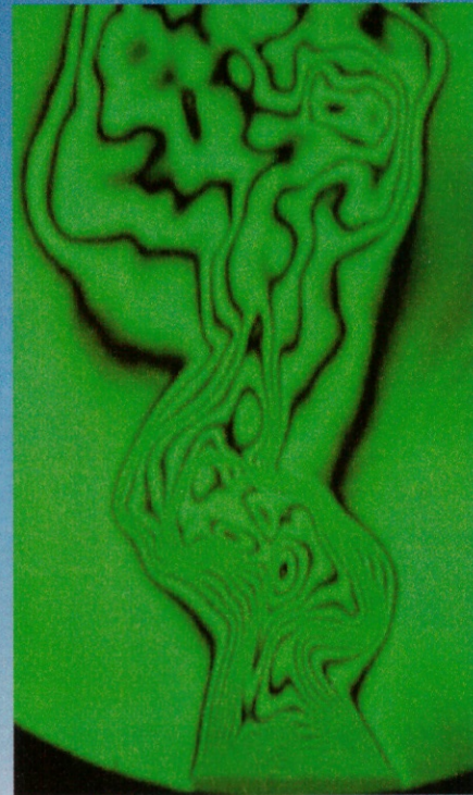
Experimental interferometric isolines of mass density (Helium d = 4.6 cm) (Schönbucher)
