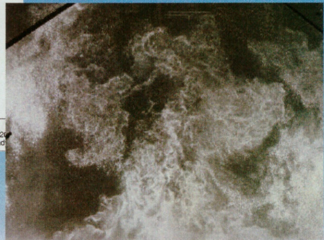
Experimental PIV images (SNL) (Helium d = 1 m)
