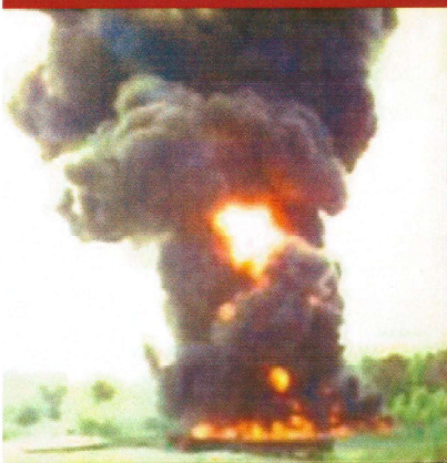
kerosene pool fire ( d = 25 m)
