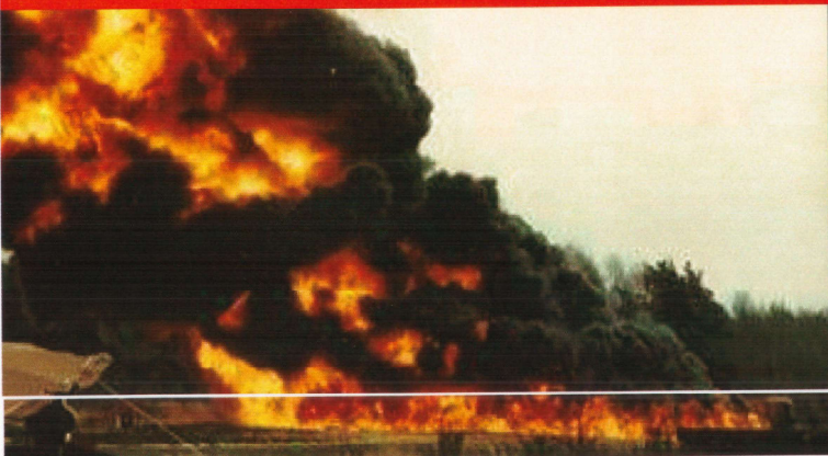
Luminous band; n-pentane pool fire ( d = 25\text{ m} )
